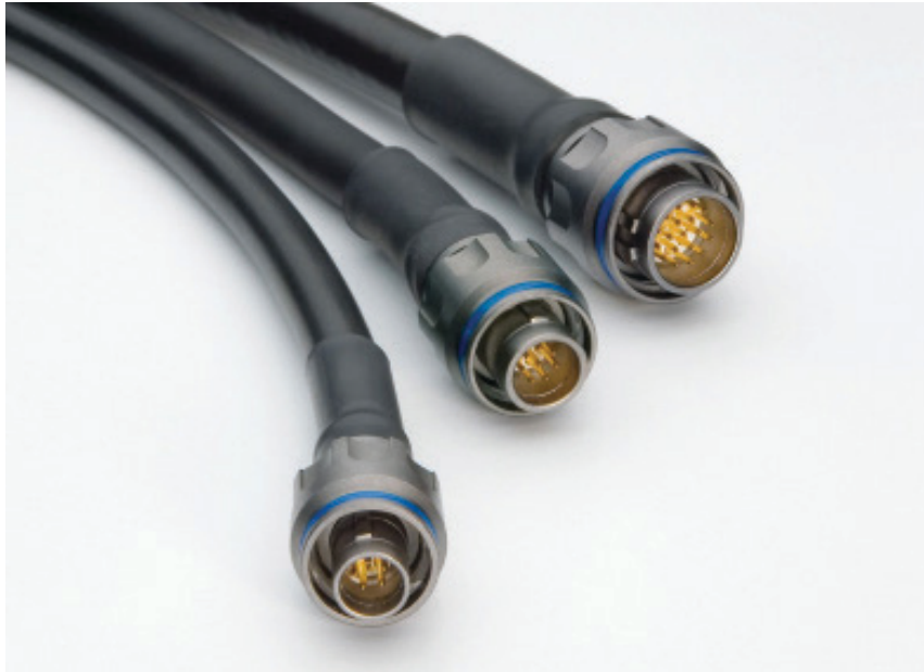
LEMO's M Series uses a stepped ratcheting coupling mechanism that tends to tighten in high-vibration applications.
