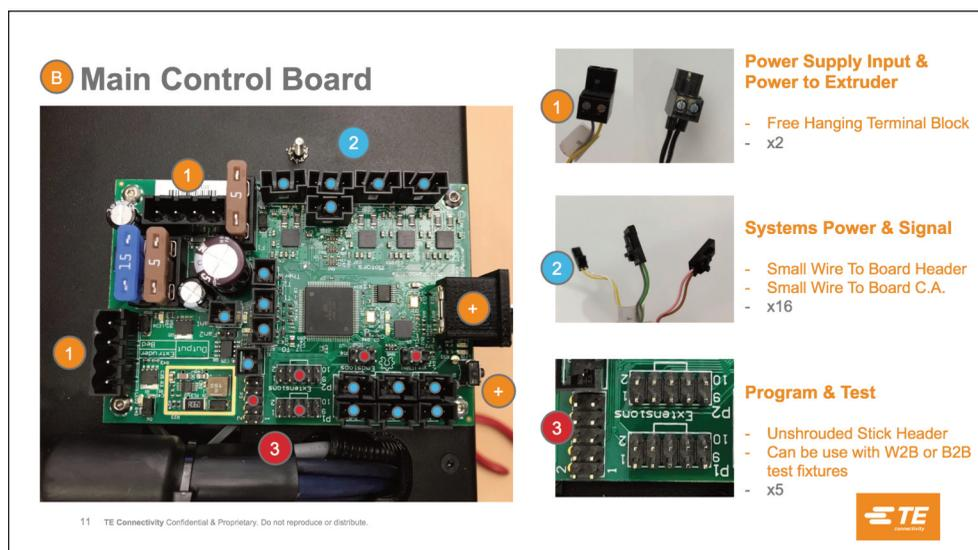
**Figure 2: Main control board components of the printer.**
