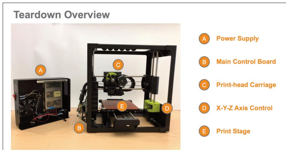
Figure 1: Overview of the desktop 3D printer.
